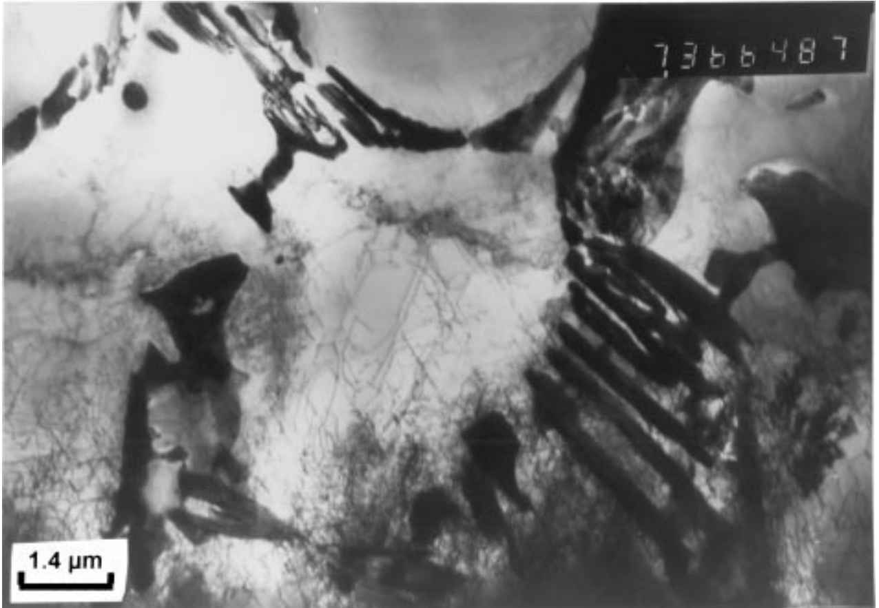
Figure 5 TEM micrograph of single layer Colmonoy coating applied with a table velocity of 1.1 cm/s. The micrograph shows a secondary dendrite arm with dislocations in the metal matrix. Further, the eutectic structure of the interdendritic part is recognisable and has a lamellar spacing of the order of 0.1 \mu\text{m} .
