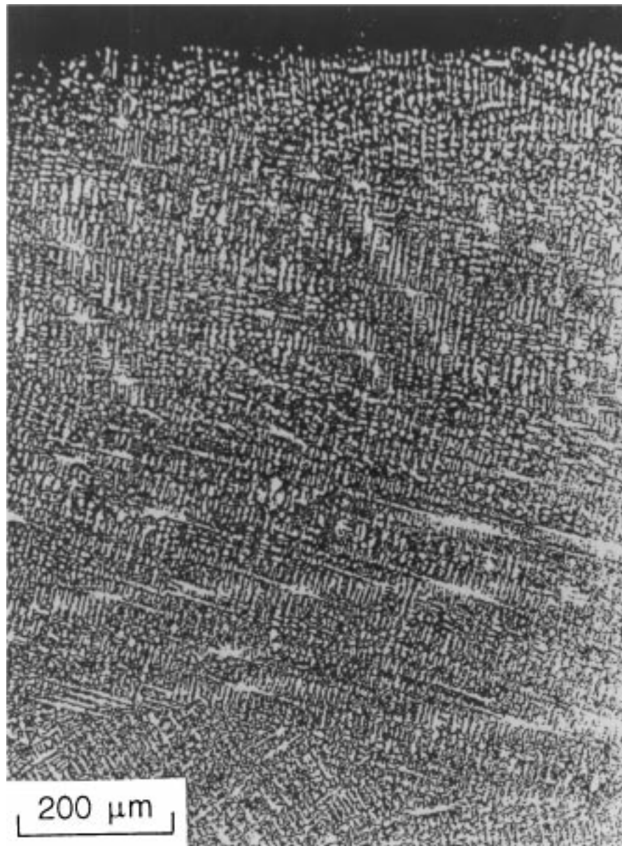
Figure 3 Optical micrograph of a cross section of the three layer coating (table velocity 1.1 cm/s) at the top of the coating.
